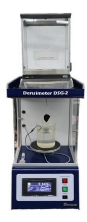
When determining density, balances are used to calculate the mass of substances in air and liquid solutions. Based on the measured values, the density is calculated.
