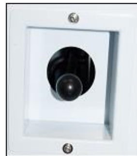
Lever arm is used to hold sample on the holder
